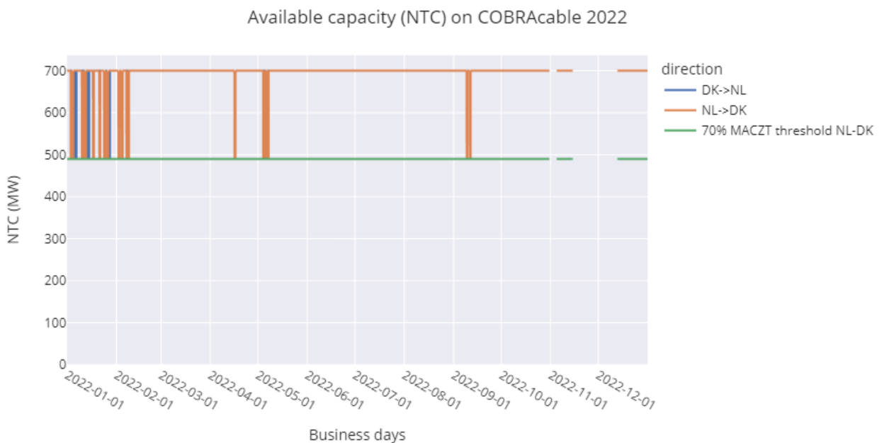
Figure 26: Available capacity (NTC) on the NL-DK1 bidding zone border. Outages are filtered out of the dataset. Period Jan-Dec 2022
