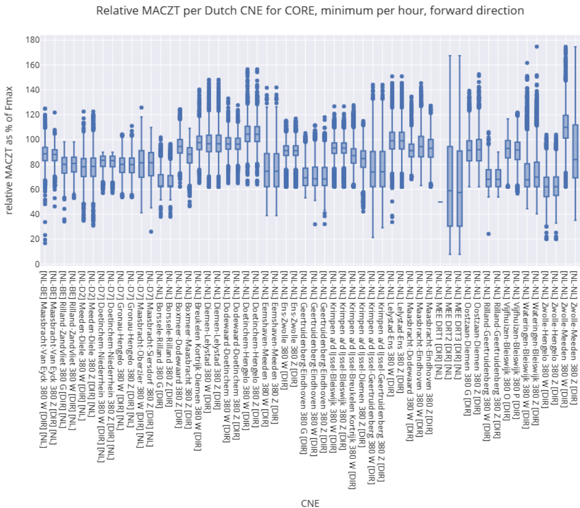
Figure 8: Relative MACZT per Dutch CNE included in Core CCR in the forward direction, based on the lowest relative MACZT per CNE per hour.
