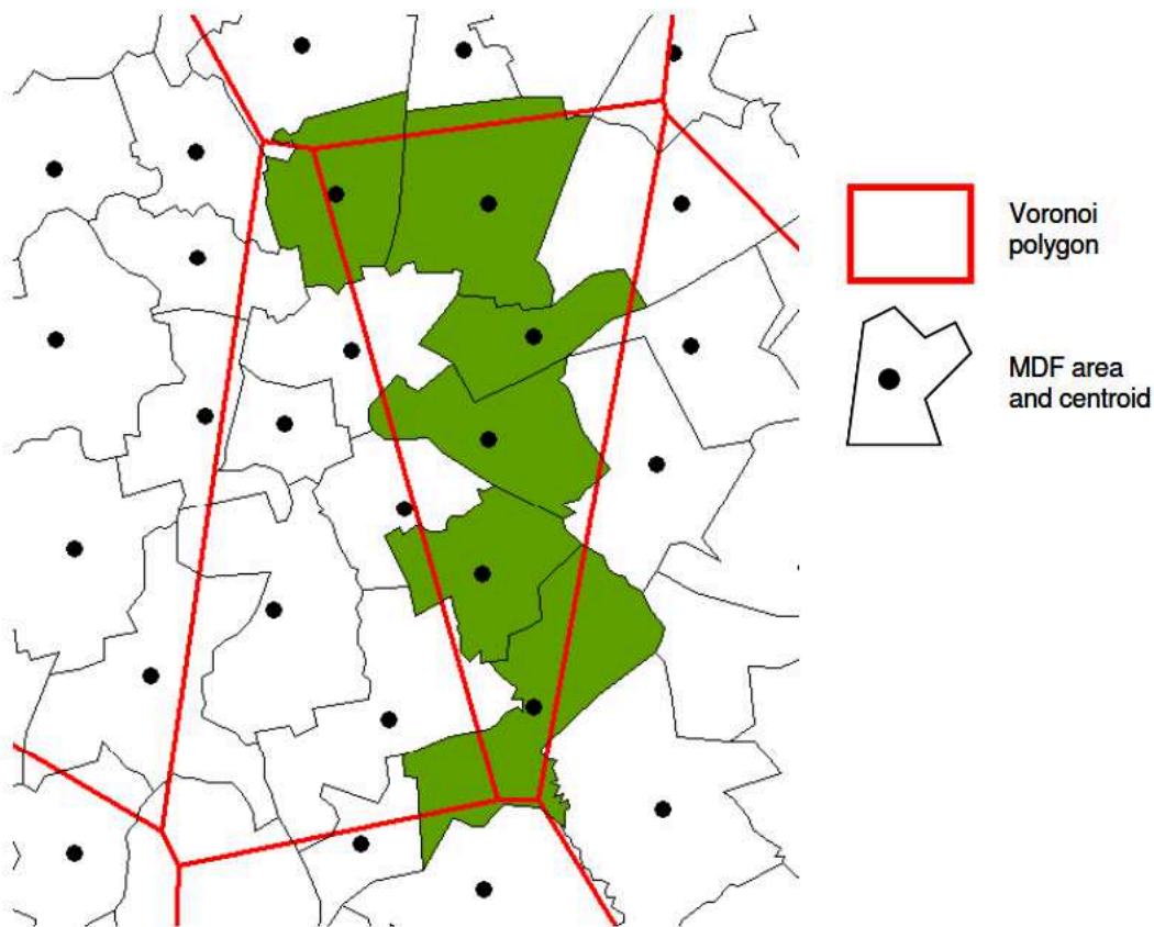
Figure A.1: Allocation of MDF areas to Voronoi polygon associated with each MCL (the green MDF regions are those allocated to the MCL with the associated Voronoi polygon) [Source: Analysys Mason]
