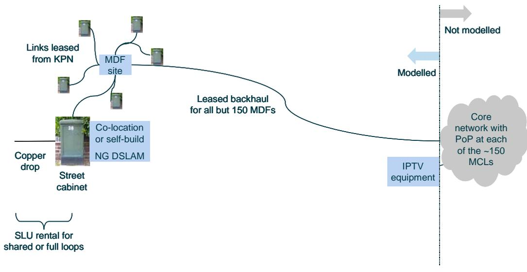
**Exhibit 3.8:** Network architecture modelled for SLU at MDF using KPN for SDF–MDF links
