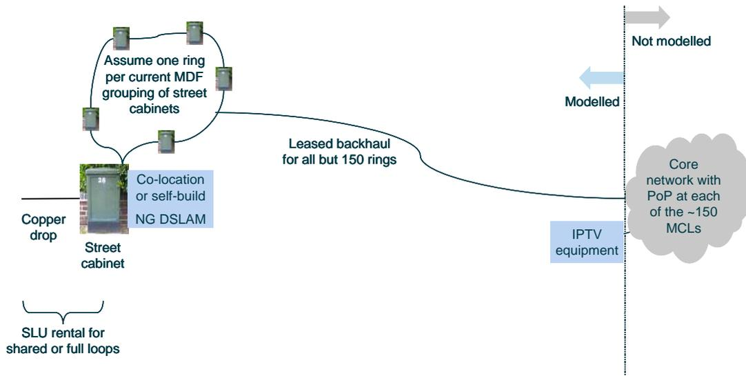
**Exhibit 3.7:** Network architecture modelled for SLU at MDF using new build for SDF–MDF links [Source: Analysys]
