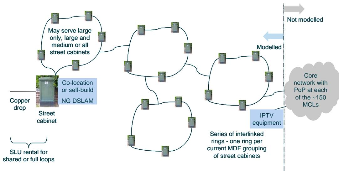
**Exhibit 3.9:** *Network architecture modelled for SLU at MCL using new build for SDF–MDF links [Source: Analysys]*
