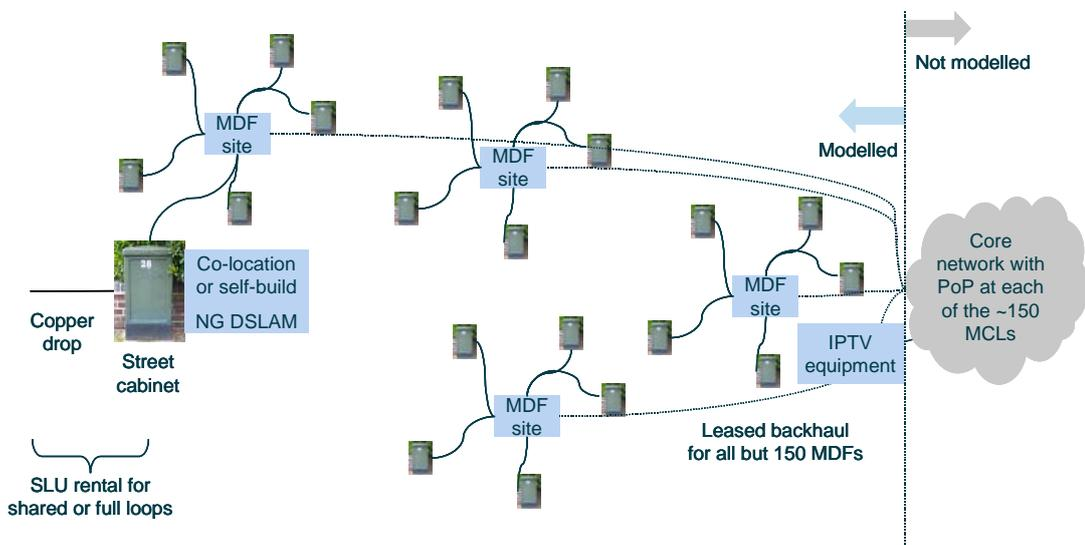
**Exhibit 3.10:** Network architecture modelled for SLU at MDF using KPN for SDF–MDF links
